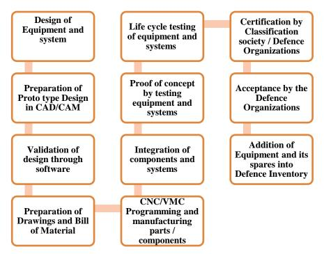
We have built our design and engineering department and ventured into complete system integration. In the above process products are prototyped, developed, functionally tested, validated, environmentally tested in compliance with stringent requirements of the Defence and Nuclear Industry. We have separate division that undertakes repairs and overhaul of valves and equipment delivered by us.
