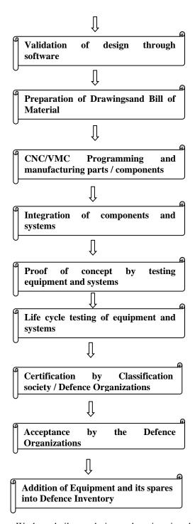
We have built our design and engineering department and ventured into complete system integration. In the above process products are prototyped, developed, functionally tested, validated, environmentally tested in compliance with stringent requirements of the Defence and Nuclear Industry. We have separate division that undertakes repairs and overhaul of valves and equipment delivered by us.
